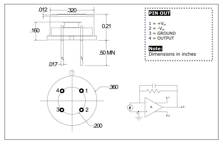
**Note:** The preamplifier portion of this receiver is a transimpedence current to voltage converter. Its output voltage is proportional to the input signal current: Application
