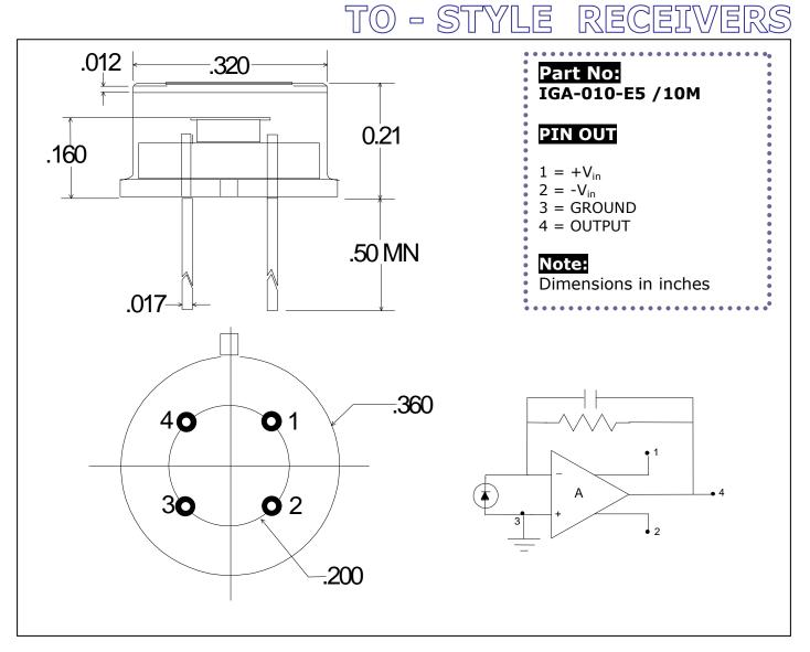
**Application** Note The preamplifier portion of this receiver is a transimpedence current to voltage converter. Its output voltage is proportional to the input signal current:
