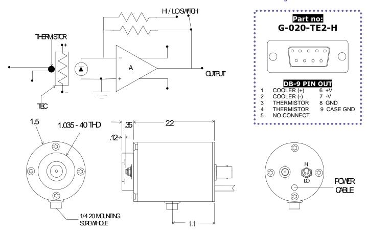
This unit is a high performance photodiode/receiver operated with a thermoelectric cooler for stabilization/cooling with a dual gain FET input transimpedence amplifier. The output voltage is proportional to the input signal current::  $V_{out} = I_{signal} \cdot R_{f}$ . The PD/AMP is a DC coupled dual gain system. Care should be taken in shielding the unit from stray light during operation to prevent saturation of the amplifier (and potential failure).
