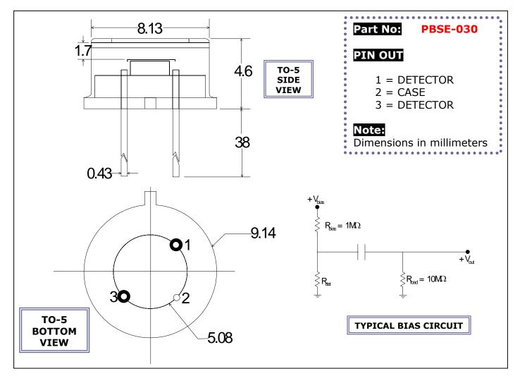
**Application Noce ELECTRO OPTICAL SYSTEMS** offers room temperature and thermoelectrically cooled photoconductive detectors. The units have state-of-the-art sensitivity and may be supported by accessories such as optical filters (longpass and bandpass), integral preamplifiers, temperature controllers and infrared source assemblies. These units find applications in industrial control systems, gas analyzers, thermal sensors, and general infrared instrumentation.
