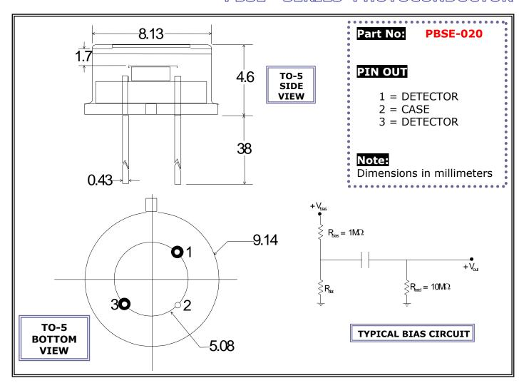
**LOS** offers room temperature and thermoelectrically cooled photoconductive detectors. The units have state-of-the-art sensitivity and may be supported by accessories such as optical filters (longpass and bandpass), integral preamplifiers, temperature controllers and infrared source assemblies. These units find applications in industrial control systems, gas analyzers, thermal sensors, and general infrared instrumentation.
