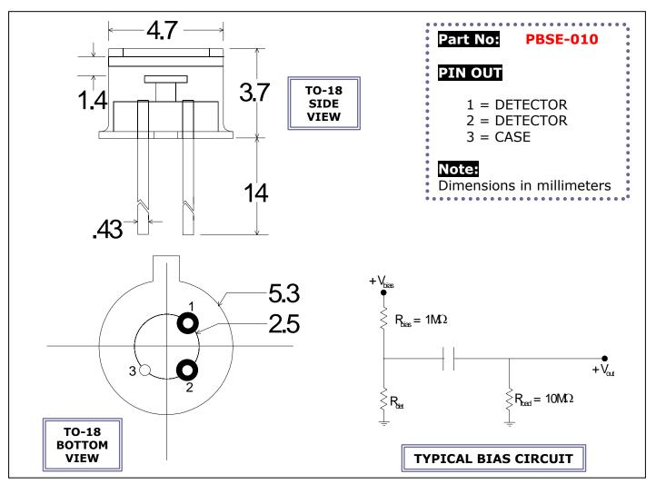
**Application** Noce ELECTRO OPTICAL SYSTEMS offers room temperature PbSe photoconductor detectors for operation in the 1.0 - 4.5 μm spectral range. The units have state-of-the-art sensitivity and may be supported by accessories such as optical filters (longpass and bandpass), integral preamplifiers, and infrared source assemblies. These units find applications in industrial control systems, gas analyzers, thermal sensors, and general infrared instrumentation.
