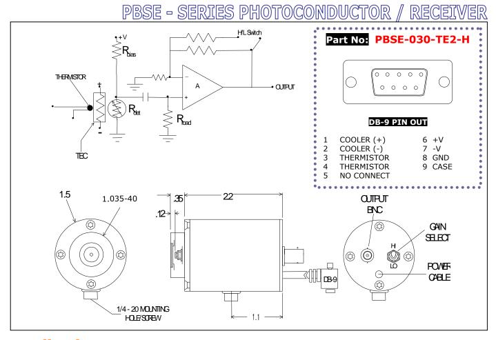
**Application** Note This unit is a high performance photoconductor/receiver operated with a thermoelectric cooler for stabilization/cooling with a dual gain voltage amplifier. The detector's bias voltage is linked to the amplifier power supply and no additional biasing is necessary. The PC/AMP is an AC coupled, dual gain detector system requiring a modulated input signal for operation.
